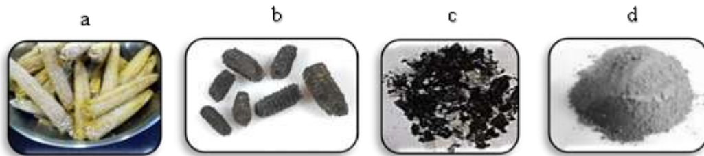
Fig. 1. Corn cob ash (CCA) preparation sequence
